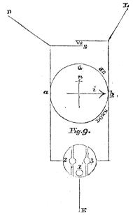
meter G. 1, 2, and 3 show in one-third size a brass disc divided into three parts, and fixed upon a block of mahogany, insulated each from the others. The middle piece of the disc is connected by a wire with the gas- and water-pipes, and is therefore in con-
